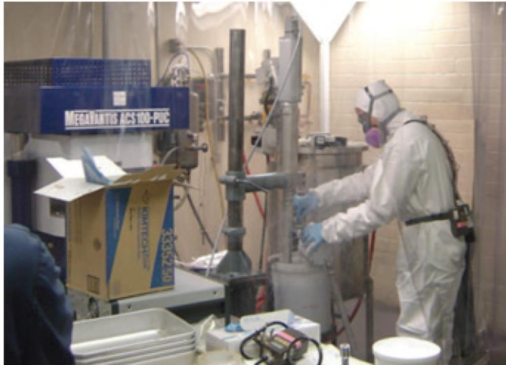
Figure 10. Nanomaterial worker wearing personal protective equipment in a work area with local engineering controls. Photo by Mark Methner, NIOSH.
